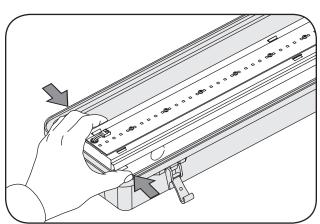
3 Squeeze the enclosure at the end and remove LED stip.
