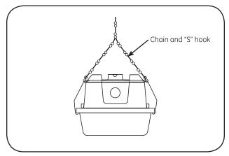
1 Mount the wrap-around brackets on the ceiling or support rail using appropriate hardware. After brackets are secured in place, install one side of the housing in the bracket, then rotate up and snap the other side of the housing into bracket. Chain and "S" hook (not included) can also be used to support the brackets
