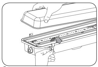
2 Unfasten the latches and remove the lens.
