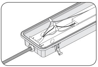
6 Connect the AC line to the black (line) and white (neutral) input wires of the LED driver using 14-18AWG twist-on wire connectors. Connect the ground wire to the green grounding wire.
