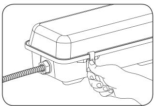
8 Reinstall the lens and secure the latches.
