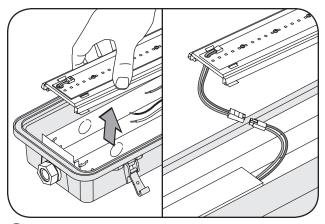
4 Lift LED strip from housing and disconnect from the LED driver.
