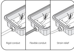
**5** Connect a rigid conduit or flexible conduit or strain relief and feed the AC line wire through the fitting.
