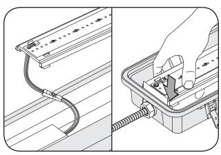
Reconnect similarly-colored wires from LED driver to LED strip. Then reattach the LED strip making sure the two end clips are properly engaged.
