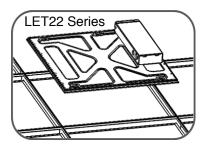
2 Insert luminaire into T-bar ceiling grid. Unit should not move freely within the ceiling grid. To ensure a consistent appearance, align fixtures in the same orientation throughout the ceiling pattern.
