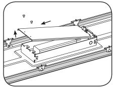
Remove electrical enclosure cover. Carefully remove knockout for AC line input wires. Install listed electrical fittings in the knockout holes for wire protection.
