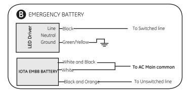
**3** Option for Step 2: Follow diagram A for 0-10V or diagram B for EMBB. Run wires from controller through a different knockout than the AC input wire. At output side of fixture, make appropriate connections using twist-on wire connectors. Follow lighting controller and IOTA EMBB installation instructions.
