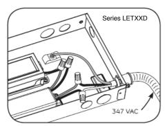
Connect the AC line to the black (line) and white (neutral) input wires of the LED driver using 18-14 AWG twist-on wire connectors. Connect the ground wire to the green grounding screw. When connecting dimming controller, wires must run through a separate knockout hole equipped with an appropriate wire restraint or cable gland.
