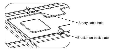
3 Bend the brackets on the back plate to make sure they hook to T-Bar.
