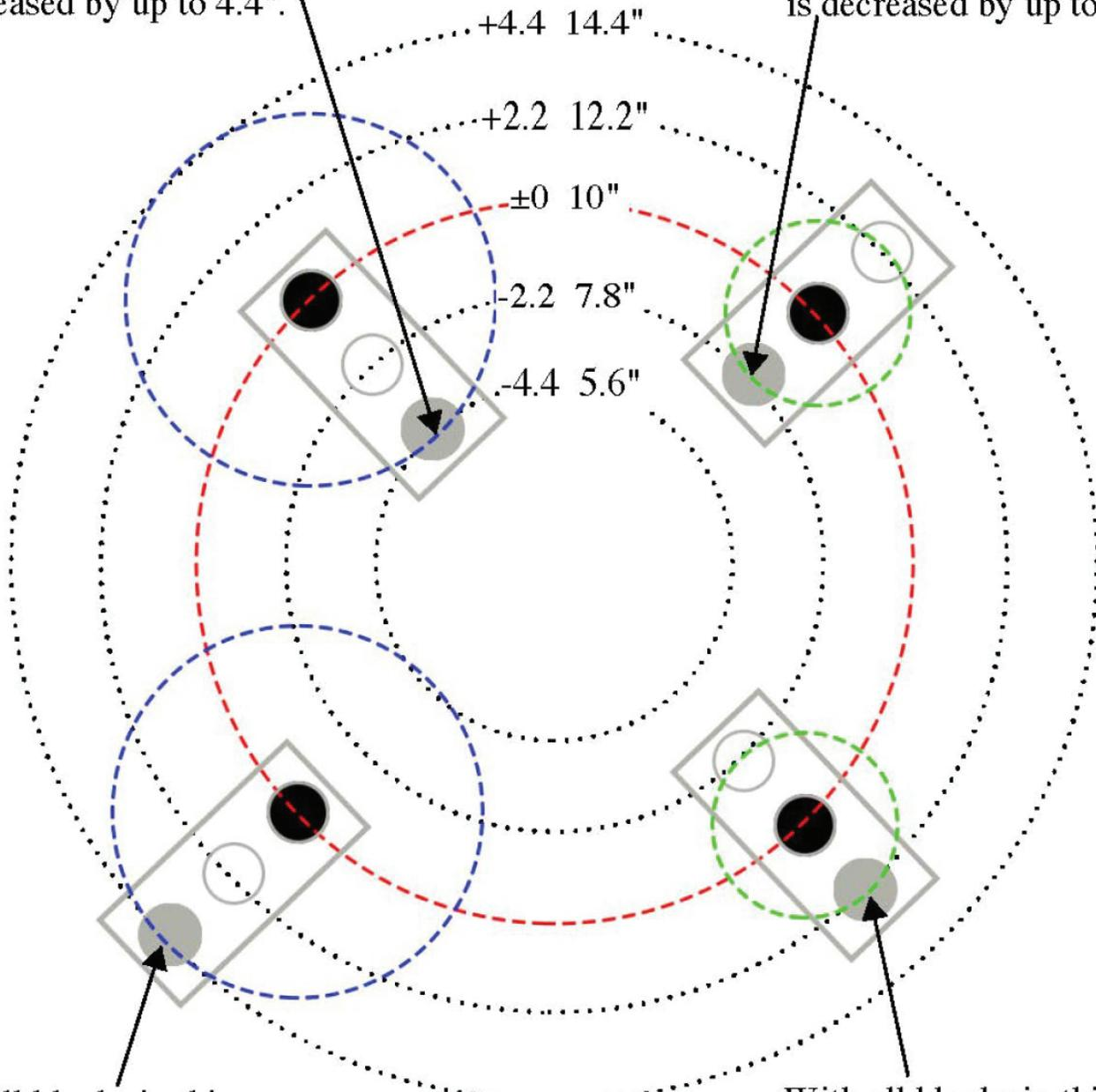
With all blocks in this configuration, the bolt circle is increased by up to 4.4".
