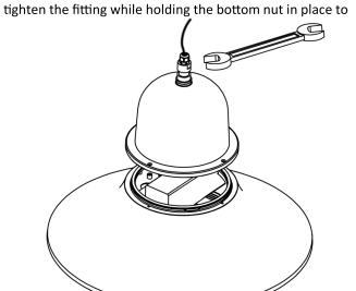
④ Once both top and bottom hardware are secure, place upper dome onto fixture and screw in hardware to reconnect.
