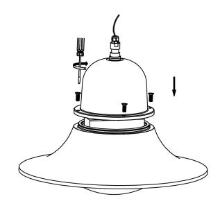
⑤ Turn the fixture over and place the clear dome over the LED assembly, and secure with the provided screws.
