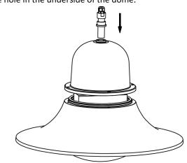
Insert the threaded fitting over the top of the cable and push the threaded end into the dome. Pull the cable taut and feed the washers and nut onto the threaded insert from underneath. Hand tighten and then use an open-end wrench to tighten the fitting while holding the bottom put in place to
