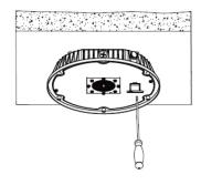
**3.** Replace the lens and check the sensor function
